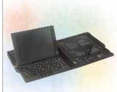
SPECIFICATIONS: Pentium III 600 MHz processor, 64 MB RAM, 10 GB HDD, integrated 10/100 Ethernet, 56K modem, 10.4 inch TFT Touch screen
